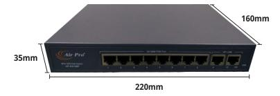
• PACKAGE DIMENSION (305mm\*185mm\*55mm, Gross Weight:1.16kg/unit
