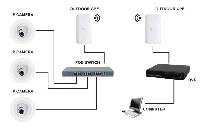
3. PTP WORKING DIAGRAM OF OUTDOOR CPE WORK WITH IP CAMERA
