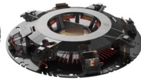
Neat cable management to reduce crosstalk
